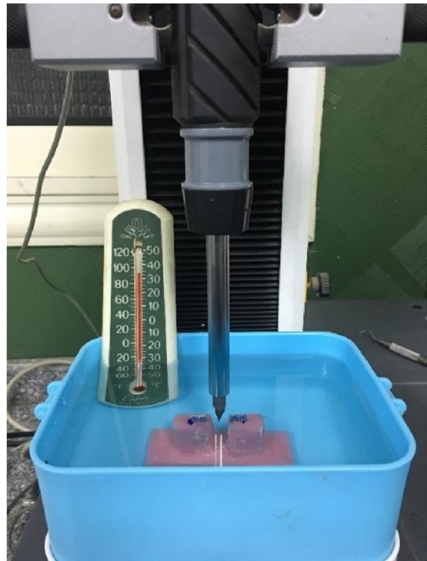
Fig. 2. Three-point bending test for orthodontic arch-wire carried out at 37 °C by placing the resin base into a water bath with controlled water temperature at 37 °C.
